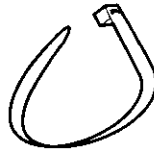
Plastic Cable Tie (shown reduced size) Qty: 1 (Recoil Start Model) Qty: 3 (Electric Start Model)
